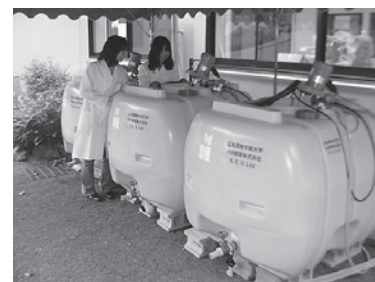
Fig. 10. Mesh bag containing SSI immobilized glass ceramic (A). Outdoor practical removal of Cs and Sr using a 1 m 3 vessel.
